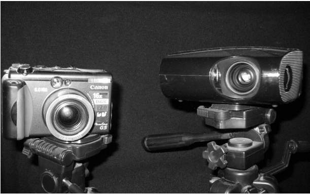
Figure 3. Camera-projector assembly. The object in the scene is fixed and it is located in the field of view of the camera and projector. In the experiments, we are using a Samsung digital projector with a resolution of 640x480 pixels, and a Canon PowerShot-G5 camera with a resolution of 640x480 in B/W.
